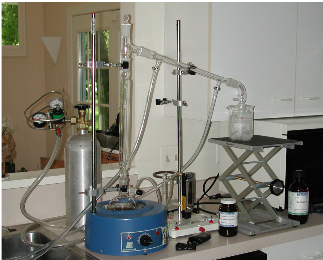
Figure 0.1 Apparatus configuration for distillation of beer samples for diacetyl analysis. Note receiver (in beaker on jack stand) is surrounded by ice. Also note carborundum boiling stones, Antifoam A and carbon dioxide flow meter. (28Jun00 - DSCN0222.pct)
